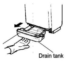
Open the drain tank cover and empty out the water.
