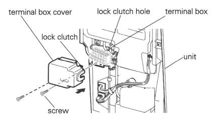
Remove the terminal box cover To gain access to the hand dryer wiring terminal block.
